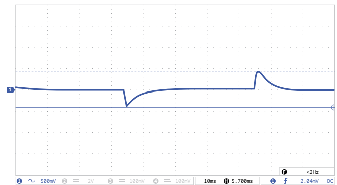
Figure 8 (d). Oscillograph chart of voltage transient deviation during load “drop/rise”.
